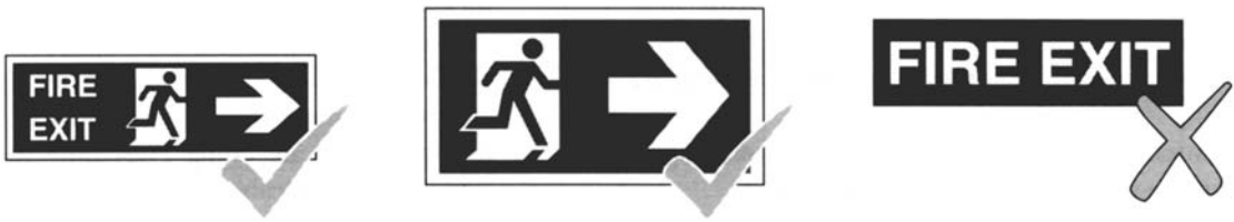
Fig. 1.12 Text only safety signs do not comply.
