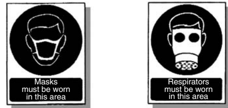
Fig. 1.11 Breathing protection signs.
